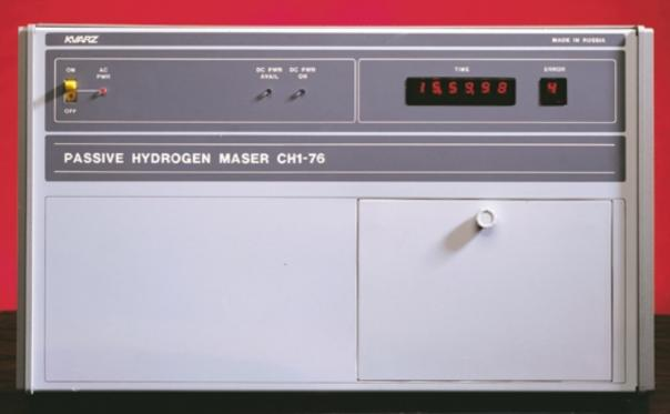
Better short & long term stability combined than Cesium □ No wear out physics package □ Half Lifetime COA of Cesium □ Long Lifetime □ Unique - the only Passive Hydrogen Maser available IEM Kvarz - world's largest producer of Hydrogen Masers
